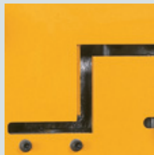
3 ANGLE STATION Cropping angle iron is possible for every angle between 45° and 90°, both internal and external.
