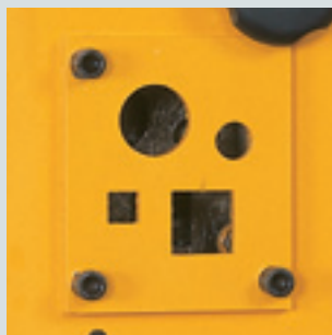
2 SECTION CUTTING STATION While cropping round and square solid bars in the standard setup, this station also allows optional blades for cropping channels, beams, Tee- and many other special profiles.
