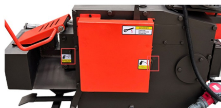
Figure 5.1: Greasing points (marked with red boxes)
