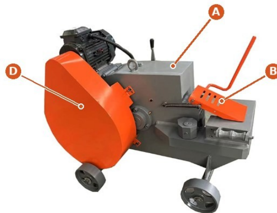
Figure 1.1: Guards and protective devices
