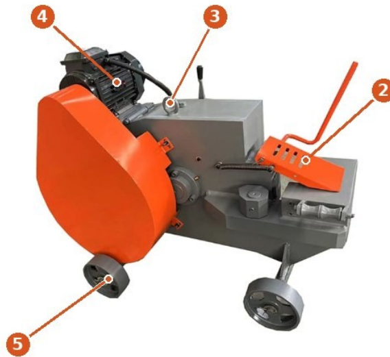
Movable guard (2), lifting eyebolt (3), motor (4), wheels (5). Main switch (1) is shown in Figure 4.1.
