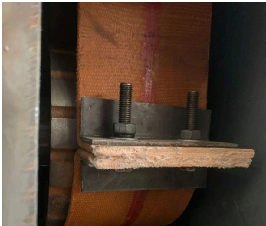
Figure 11 - Belt retaining bracket detail
